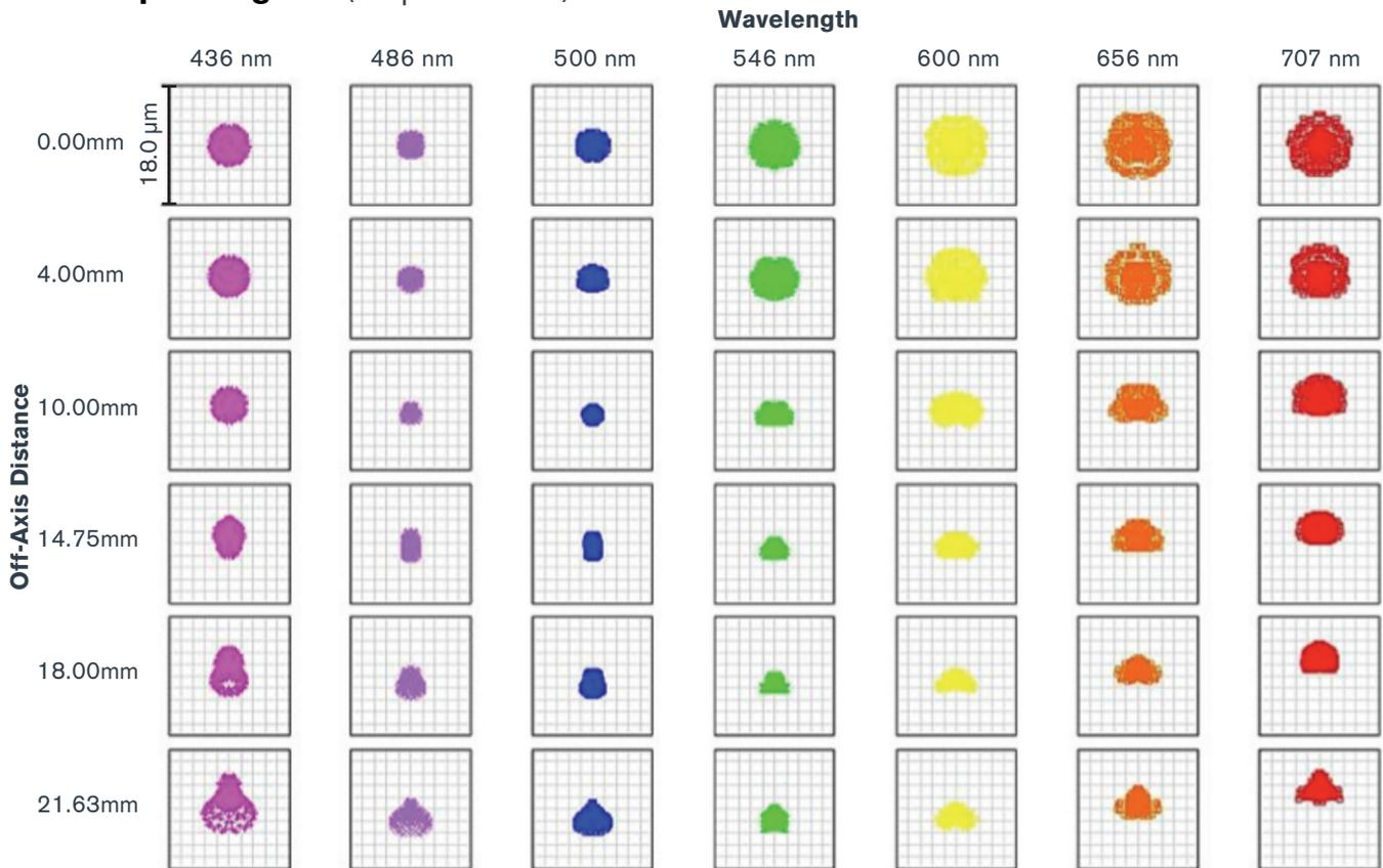
Fig. 10: The RASA's matrix spot diagram reveals that it forms remarkably tight star images across the entire visible spectrum from deep violet (430 nm) to near infrared (700 nm), from the center of the field to more than 21mm off axis. In practice, a field of view 52mm diameter is practical. The boxes are 18 microns on a side.
