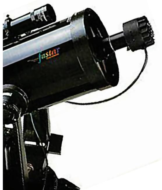
Fig. 6: The 8-inch f/2 Fastar carried a PixCel CCD camera ahead of the corrector plate. In a fast telescope, it turns out that the best place for a compact image sensor is at the prime focus.
