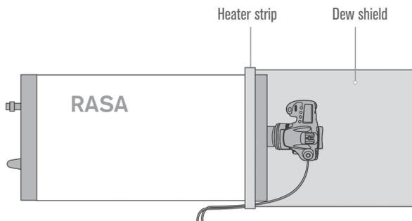
Fig. 20: The dew shield serves three important roles: 1) it prevents dew from forming on the corrector plate, 2) it shields the camera from stray light that can be reflected into the RASA, and 3) it prevents skylight outside the field of view from reducing image contrast.
