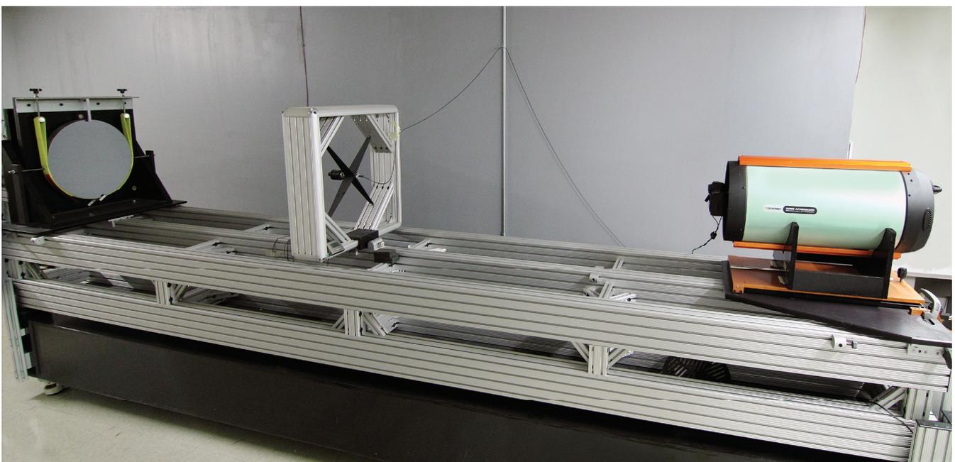
identical.” If the corner images are not as sharp and tight as the center image, the tilt of the correcting lens assembly is adjusted so the on-axis and off-axis star images appear sharp at the same focus point. “When a RASA leaves the factory, it’s in good alignment,” said Kopit. “Although the user can adjust the tilt of the correcting lens assembly, it’s usually not necessary.”
