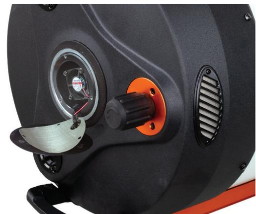
Fig. 14: The 12VDC MagLev fan along with improved venting allows for good airflow within the optical tube. This helps cool the telescope to ambient temperature.
