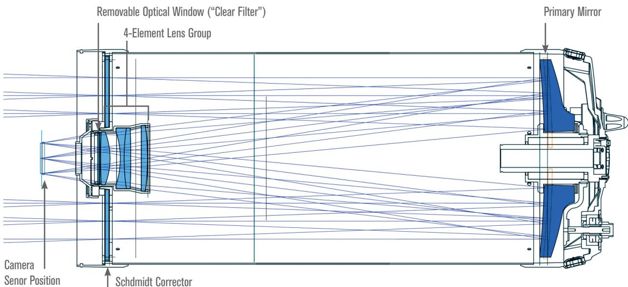
Fig. 9: Celestron's Rowe-Ackermann Schmidt Astrograph consists of a Schmidt corrector plate, primary mirror, and a four-element corrector lens. Light enters from the left, passes through the corrector plate to the primary mirror, then reflects back through the corrector lens and comes to focus in front of the corrector lens.
