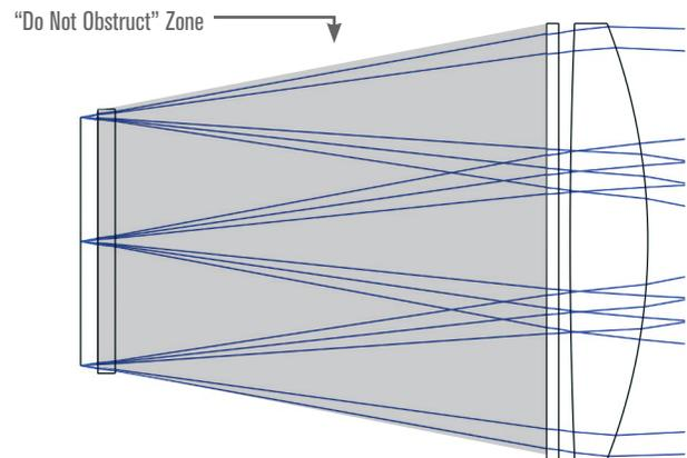
Fig. 17: The “Do Not Obstruct” zone is the region between the corrector lens and the image sensor. Anything that obstructs light passing through this volume causes light loss.
