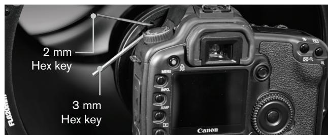
7. If the star pattern is thin on one side, adjust the collimation screws so that the star moves towards the thin side, then adjust the position of the astrograph to re-center the star. Repeat this until the defocused star image is concentric.
