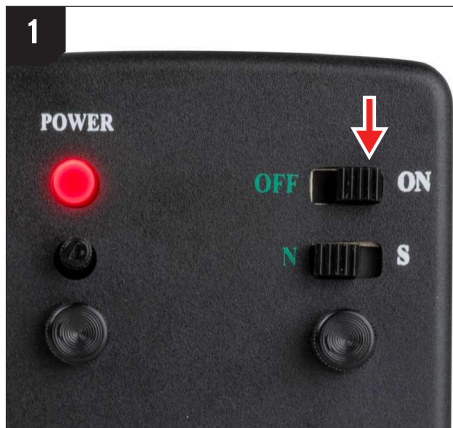
1 Slide the On/Off switch (I.) to the "On" position. A red LED will illuminate.
