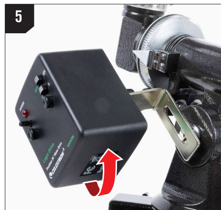
5 Align the slotted hole on the motor bracket with the threaded hole where the Allen screw was. If necessary, pivot the RA worm shaft by rotating the connected motor drive. This will rotate the shaft until the slotted hole in the bracket aligns with the threaded hole on the mount.
